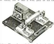
position. The relay, which is of the double-pole, double-throw type, is practically free from hum and has absolutely no chatter or bounce in the contact arm, according to the manufacturer's statement. Among its uses are antenna change-over, multi-band tank switching, and 60 cycle power switching. Uses but 5 watts on 110-volt, 60 cycle A.C.
