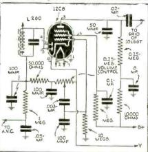
Alternative 2nd Detector-First A.F. stage, using 12C8 tube instead of Westector and 12SJ7.
