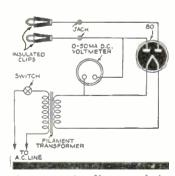
plates and the filament of the tube. In this way, the A.C. output is rectified so that it can be read on the meter. The greater the sensitivity of the meter, the better the results.—Ralph Scott.
