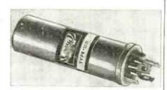
A special ventilating system allows internal gases to escape, but prevents air from entering, and a bakelite terminal base is used that completely eliminates leakage. Internal construction is all aluminum and electrolyte cannot come into contact with any corrosive metal.
