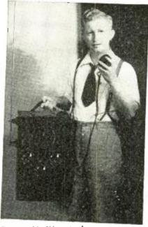
The portable 21/2 meter ★ transceiver—it carries 2-way phone.
