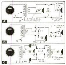
The diagrams show three methods of connecting an extension loud speaker.
