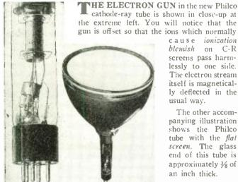
cathode-ray tube is shown in close-up at the extreme left. You will notice that the gun is offset so that the ions which normally
