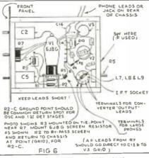
Bottom view, showing how 6J8G tube is mounted, also disposition of the other parts.
