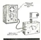
can be used in matching I.F. coils, by tuning the radio to a strong harmonic of the oscillator frequency.—Frederick F. Slack.
