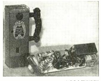
Here we have a peek at the "innards" of the miniature radio transmitter built into a talcum powder can. It is self-contained, oper-ates from batteries, and so may be carried about freely.
