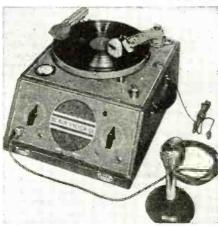
The portable model records and reproduces 10-or 12-inch records at 78 r.p.m., using the outside-in method of recording. It is complete with am-plifier, loudspeaker and visual indicator.
