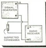
Hook-up for Testing Condensers. No. 1193.
