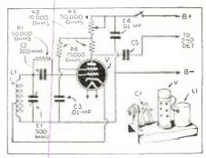
Circuit diagram for a simple and very useful beat-frequency oscillator, which will make it easy to locate those elusive DX stations.
