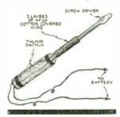
hold a bolt or a screw for insertion in an out-of-the-way corner. Of course, the tool will not operate with brass screws.—
