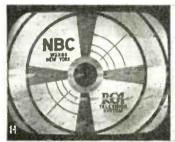
Fig. 11. Excessive auto ignition interference.
