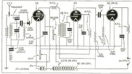
A 3-tube portable battery receiver using Megadyne crystal hook-up.
