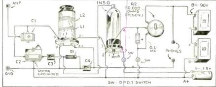
The famous "Oscillodyne" circuit brought up to date-using the new 1.4 volt tube, Type INS-G.
