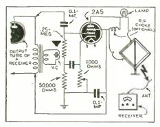
Audio frequency transmission with a loop antenna.
