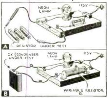
Top-Useful continuity testing device for the experimenter. Below-Simple tester for condensers.
