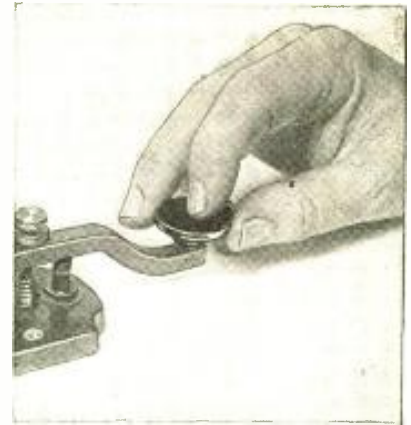
The grip on the radio key should be light; the position of the thumb, also the first and second fingers is shown above.
