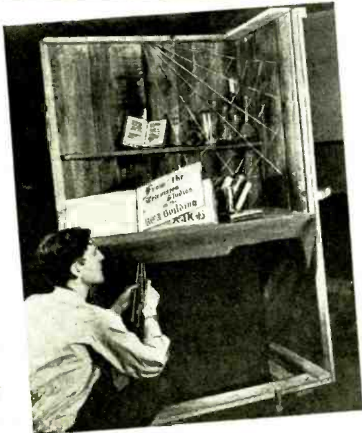
Left—How book leaves are turned for a television presentation over the NBC system. Each leaf is turned by means of a wire projecting down through the shelf and out of the focus of the television camera. Note the artistic spider-web effect used in this setting.
