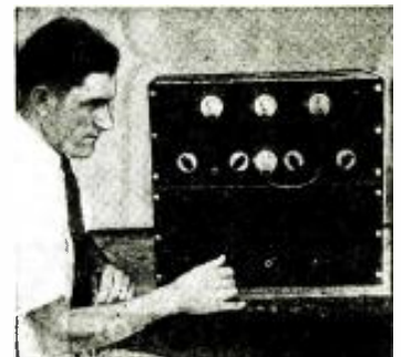
Here is a photo of the modulator to be described by Harry D. Hooton, W8KPX, in the October number. It is especially designed for use with low-powered transmitters.
