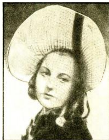
This picture was reproduced via radio, 100 lines per inch, at a speed of six square inches per minute.
