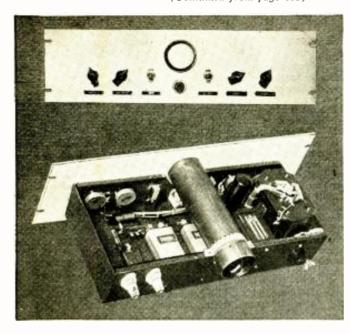
primary keying is now employed. With the use of this type of keying the final ampli-fier power supply does no work until the key is depressed, even though the "HV" switch has been closed. The keying relay (5) is operated on low voltage, about 6.5 V. to be exact, so that contact with the key or its leads will cause no inconvenience.
