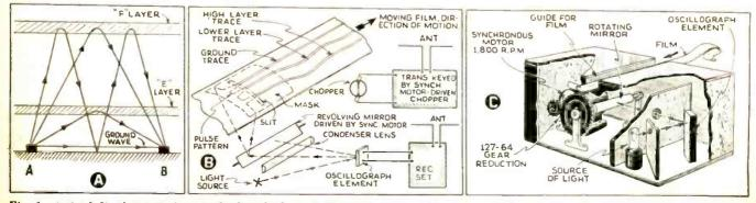
Fig. 1, at the left, shows various paths by which an S-W signal may arrive at a receiving station. Center, schematic diagram of system used with automatic layer-height recorder. Right—The assembled recorder with film driver and film container omitted.
