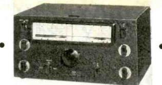
Lett—The handsome cabinet with folding doors houses one of the new de luxe 20-tube Midwest chassis. Tuning is greatly simplified by the large illuminated dial; 3 loudspeakers provided. New "communications" type receiver, the National model NC-80X. This IO-tube receiver has erystal filter and it covers the "broadcast" station band, and also the "short-wave" bands.
