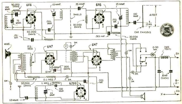
Wiring diagram of 5-meter mobile set.
