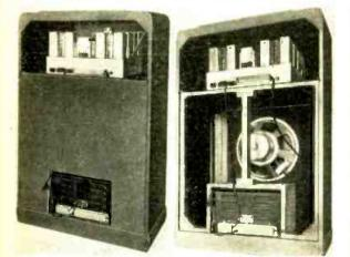
Left—Rear view of the speaker compartment; back in place. Right—With back removed.
