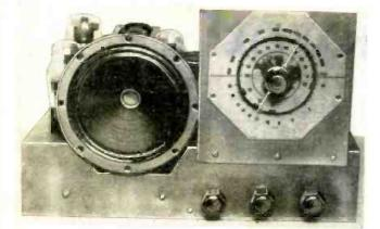
Front view of the 5-T receiver, which may be arranged for tuning in 5 meter phone by the simple addition of two tubes.
