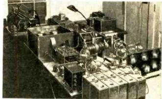
Fig. 3. A preliminary multifrequency automatic recorder of ionosphere heights and critical frequencies, originated at the National Bureau of Standards in 1932.
