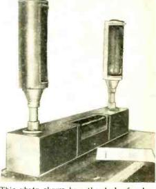
This photo shows how the desk of a lec-turer or demonstrator will look, possibly at the World's Fair (New York) two years hence. The microphone which picks up the voice is seen in the center of the desk, while at either side we see the two photo-cells which pick up the reflected scanning rays from the speaker's face.
