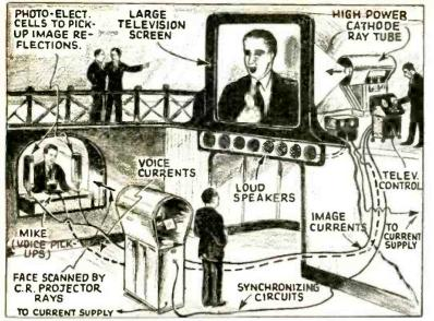
The new Telefunken television amplifier system—the scanning light illum-inates the face of the subject and photo-electric cells pick up the reflected light rays, which are amplified and passed into the cathode tube behind the large image screen.
