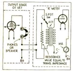
A simple circuit for constructing an "R" signal meter.
