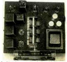
Looking down on the 6-tube superheterodyne receiver, the tube sockets being clearly visible,
