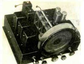
General view of the 6-tube superhet, with its calibrated dial. (No. 657).
