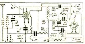
2-Tube Converter With Plug-in Coils-1093
