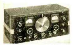
A Typical "Communications" Type Receiver-the 1938 Super-Skyrider
