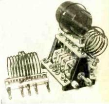
Transmitter Coil-Switch Unit.
