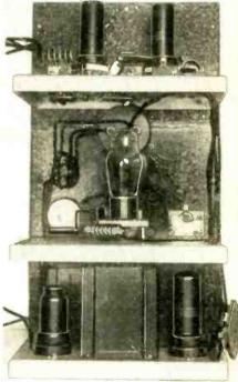
The top deck is the M.O.P.A.; center is the receiver; and bottom is the class "B" modulator,
