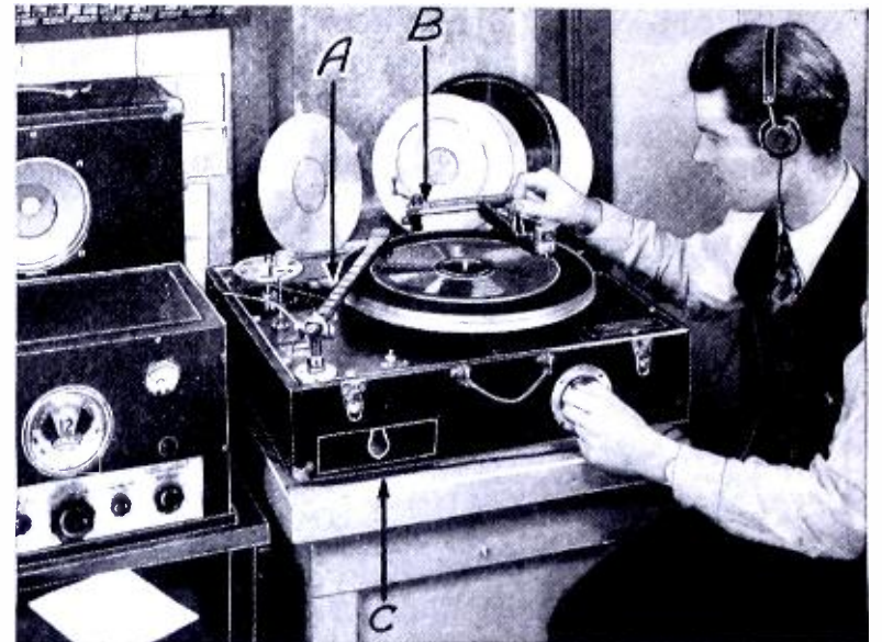
Fig. 2—Acetate High-Fidelity Recordings of "Foreign" Broadcasts being made by a Short-Wave Listener
