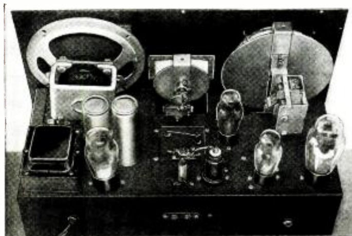
Rear view of the RSR receiver, showing the well-spaced arrangement of the parts. This set showed excellent DX-getting ability.
