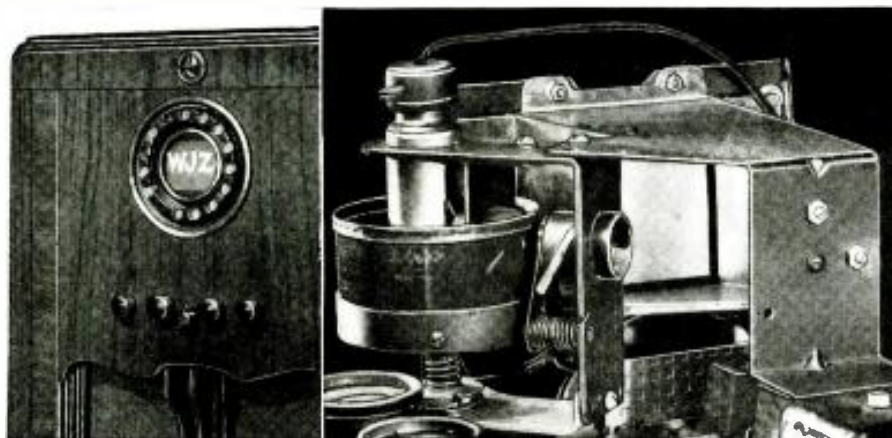
Appearance of the Movie Dial mechanism which projects greatly enlarged call-letters and frequency on a screen in the front of the radio cabinet.
