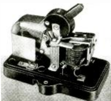
Interior mechanism of new circuit-breaker.
