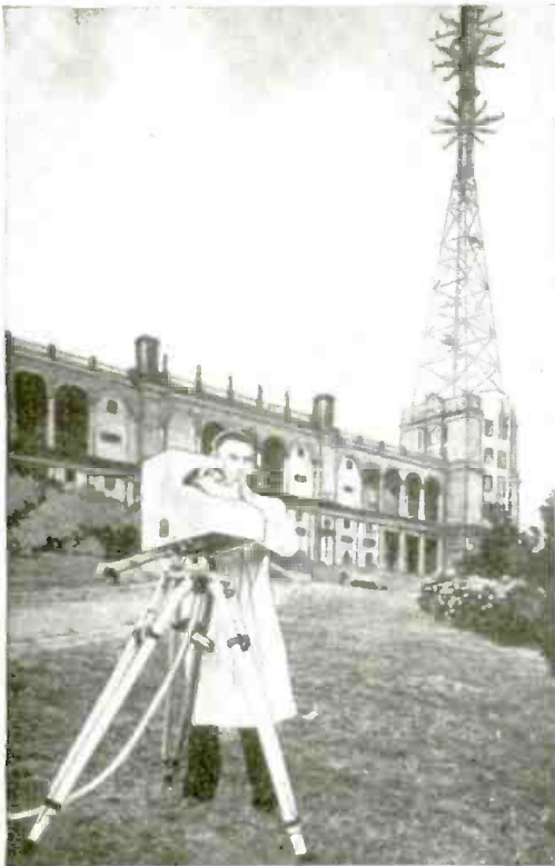
Television in England—The Marconi E.M.I. instantaneous television "camera" picking up an "outdoor" view at the Alexandra Palace. The ultra short wave aerials for transmitting the image and sound can be seen on the tower at the right.
