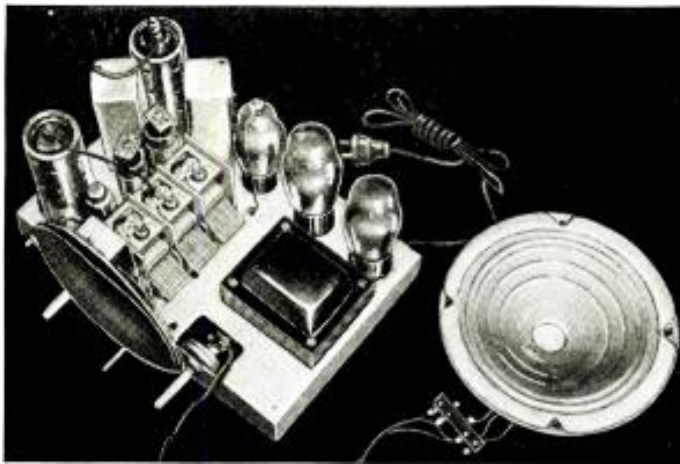
The "Super-5"—the various bands are tuned in by means of a switch.
