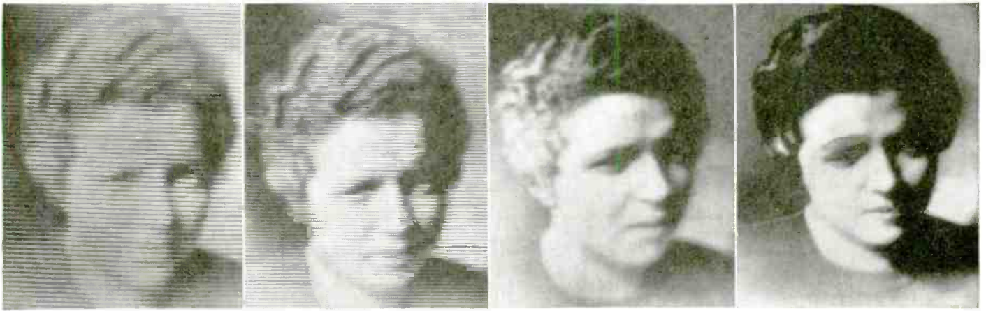
The pictures above tell in vivid fashion the story of the improvement in television scanning. The image at the extreme left was scanned with 90 lines, the next with 120 lines, the third image with 180 lines, and the one at the extreme right with the new Philips 405 line system. Note that with the 405 line scanning the lines are no longer visible. The Philco system in this country is about to experiment with 440 to 450 lines scanning, while the other companies interested in the newer system of electronic television in this country have been increasing the lineage repeatedly in an effort to obtain more perfect images.
