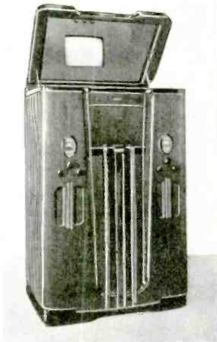
Front view of the Philco television receiver with "image" and "sound" tuning dials at right and left of cabinet.
