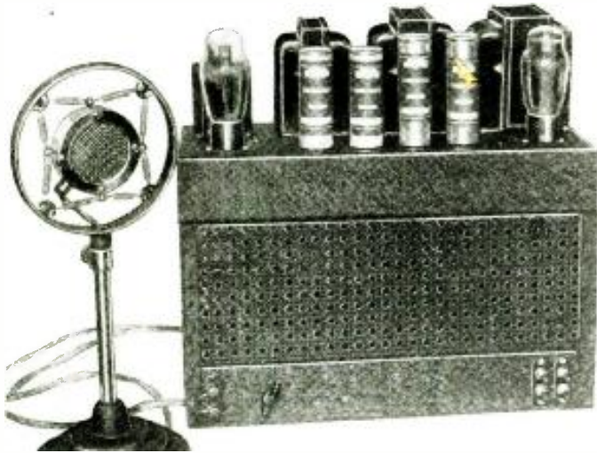
Complete modulator, including the crystal microphone.
