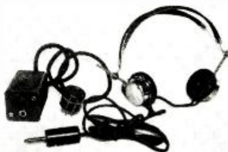
Headphone and jack which can be quickly put in operation on any all-wave receiver. When the phunes are in use the loudspeaker is cut out. (No. 538).
