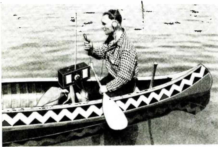
Perry Green, Maine guide, making a test of the ultra short wave transmitter and receiver which can be seen on his canoe. Guides of the State of Maine have approved the equipment for use in case of emergency where persons are lost in the woods or where accidents happen in the remote places where woodsmen travel. With this new ultra short wave equipment which can be carried on a packboard the guide can be in constant communication with the main camp or with other searching parties.
