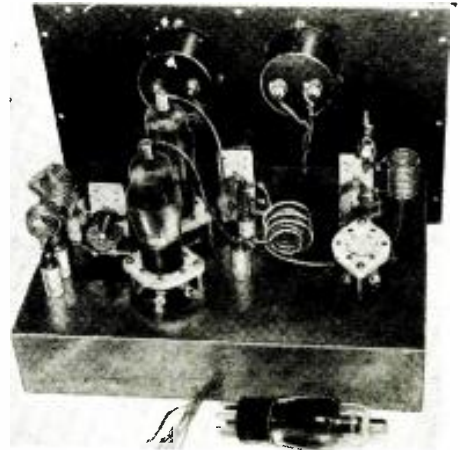
Rear view showing how the parts are placed for shortest connecting leads.
