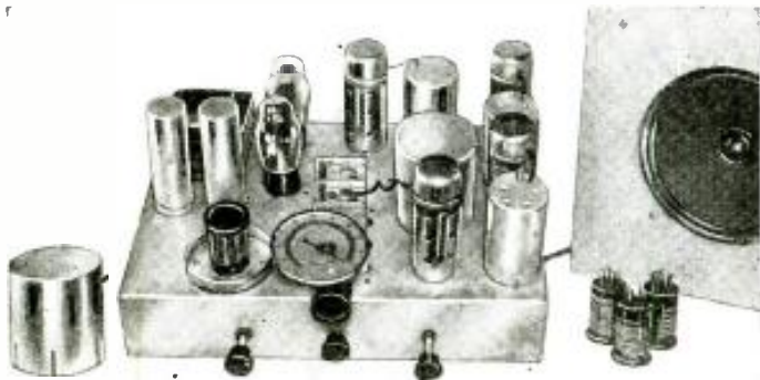
A 6-tube Dual-Wave Superhet that will appeal to many. It uses plug-in coils. No. 312
