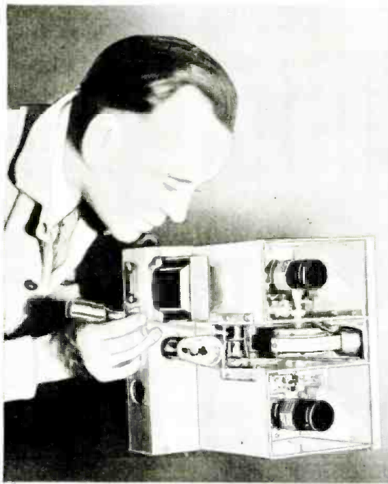
Fig. 7. No shielding is necessary for the portion of the R.F. tube between the cabinet compartments. Right: Panel view of receiver; while 5 knobs appear the instrument has single dial control. Fig. 1.
