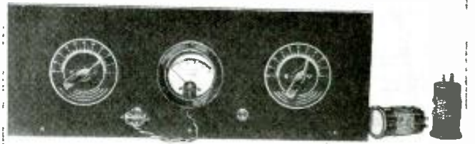
Front view of the oscillator-amplifier, which includes crystal control. This will serve as an exciter unit for the finished transmitter.
