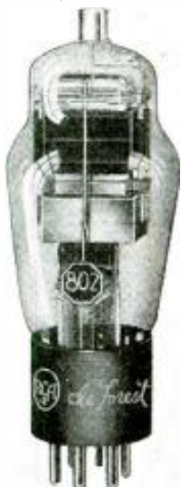
New RCA 802 screen-grid pentode for transmitters. (No. 263)
