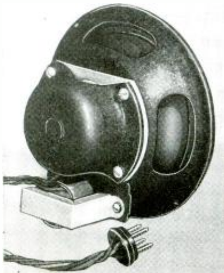
The dynamic loudspeaker specified for the "All-Star Junior" superhet, with its cord and plug.
