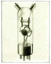
The latest practical form of Magnetron tube of German origin.
