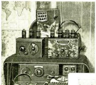
GLOBE-TROTTER: this works fine. The set on the right is a three-tube ALLEN. This works better than any of the others that I have built as yet. The one inside the cabinet is my "old faithful"—it has three tubes—35 Det., 27 and 45 output. The power supply on the right supplies the set in the cabinet.
