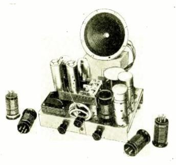
Complete "RGH-4" chassis and loud speaker, together with plug-in coils. Boy, what a wallop this set develops! And it uses but four tubes, including the rectifier.
