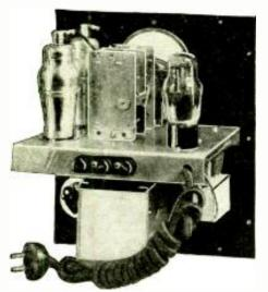
Rear chassis view of the new 2-stage Booster, No. 166.
