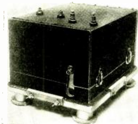
Left—Receiving set used for picking up "marker beacon" as well as "landing beam" signals.
