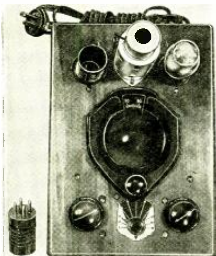
Here's a nifty short-wave converter that works on 110 volts A.C. or D.C. Plug-in coils are used for tuning in the various radio frequency bands. (No. 160)
