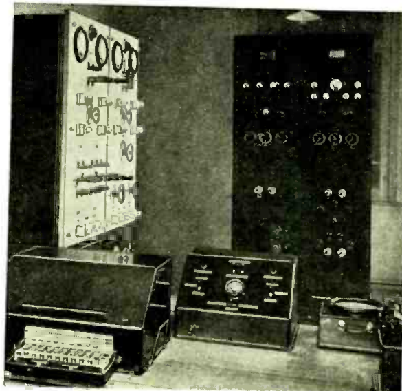
Left—view of the transmitting and receiving equipment used on the ultra short-wave link across the English channel; a teleprinter is used.
