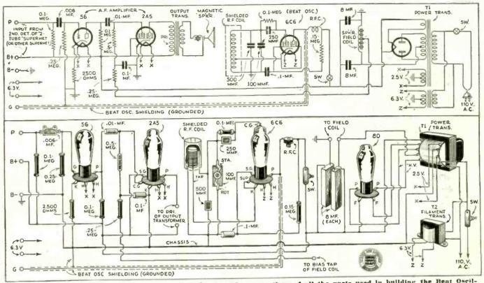
Picture, as well as schematic wiring diagrams, showing the connections of all the parts used in building the Beat Oscillator, Audio Amplifier, and Power Supply Unit here described by Mr. Mitchell, and designed for use with the "2-Tube Superhet" described in the December issue.
