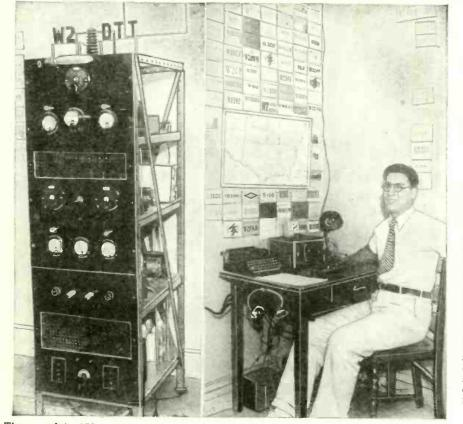
The complete 250 watt crystal-controlled transmitter owned and operated by Alvin Abrams in New York City under the licensed call of W2DTT. Mr. Abrams is observed seated at his operating desk, together with a small part of the great number of QSL cards he has received from all parts of the world.
