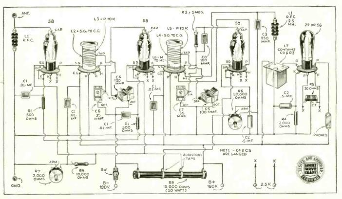
It's a "cinch" to build this dandy 4-Tube Receiver, with its exceptionally high sensitivity for yeak or distant signals, by following the picture diagram presented above. The tuning of the set is simple and it will undoubted'y make many friends.
