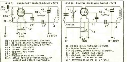
Above-diagrams with values of condensers and resistors for the frequency doubler circuit and also the crystal oscillator circuit.
