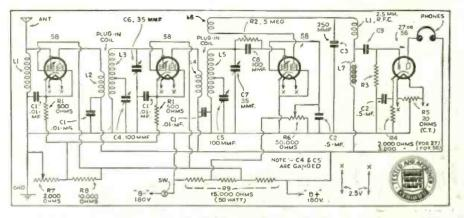
Schematic wiring diagram for the 4-tube receiver employing two stages of R.F.
