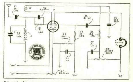
Schematic wiring diagram illustrating the general relation of the relatively few parts used in building the "19" Twinplex—a dandy 1-tuber for the embryo short-wave "fan".
