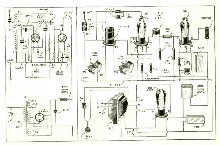
Complete schematic and picture wiring diagram, enabling anyone to build the 3-Tube Short-Wave Receiver here described. It operates on your 110 volt A.C. lighting system—no hatteries required and it will haul in the "foreign" stations like nobody's husiness.
