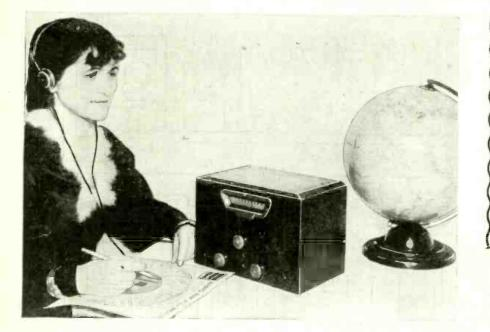
This 3-tube receiver is to be operated from a 110 volt A.C. circuit. A 58 tube is used as a detector as it is very reliable for this purpose. The detector output is fed into a 56 audio amplifier. The third tube is a rectifier. Plug-in coils are used to change the wave bands.
