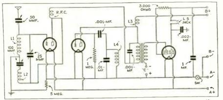
5-Meter Super-Regenerator circuit: the set-up consists of 3 tubes, a regenerative detector, a quenching tube and a pentode output tube.
