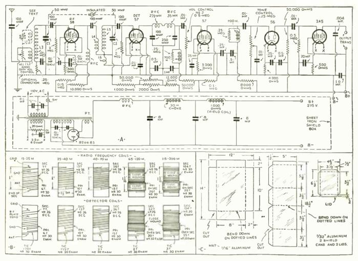
Coil data and scheme of connections for the "Advanced" 5-Tube Receiver.
