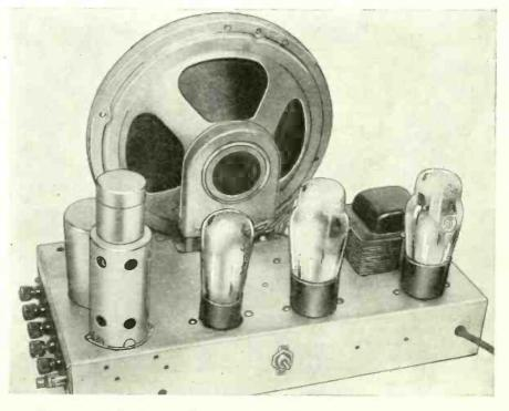
Top view of the beat oscillator, audio amplifier and power supply unit.
