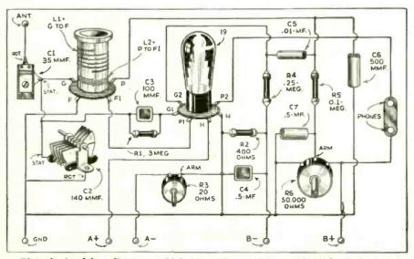
Pleturized wiring diagram which even the most inexperienced short-way fan ean follow, in order to build this excellent one-tube receiver which gives 2-tube results.
