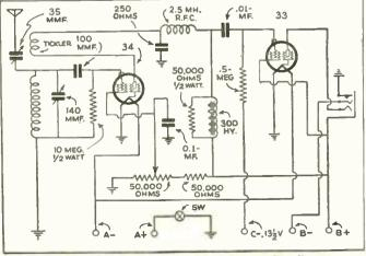
Wiring diagram of "Pretzel-Bender Two".
