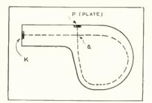
Here is a "Grid-less" ultra short-wave transmitter tube, in which the electronic current reacts upon itself. as shown by the circular dotted line.
