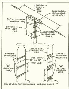
This system is extremely light in weight and no difficulty should be experienced in supporting it with the antenna wire alone. However copper antenna wire alone. However copper clad, rather than solid copper wire, is recommended because of the greater strength of copper-clad wire over solid (Continued on page 685)
