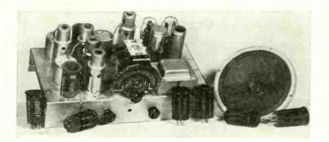
This photograph clearly shows the neat arrangement of parts used in this modern short-wave superhet.
