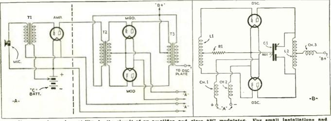
The diagrams, above, show at Fig. A-the circuit of an amplifier and class "B" modulator. For small install especially for portable sets, the push-pull oscillator circuit shown in Fig. B will find many friends.
