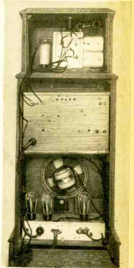
Rear view of Mr. Whisk's receiver, which contains "short" as well as "broadcast" range units.
