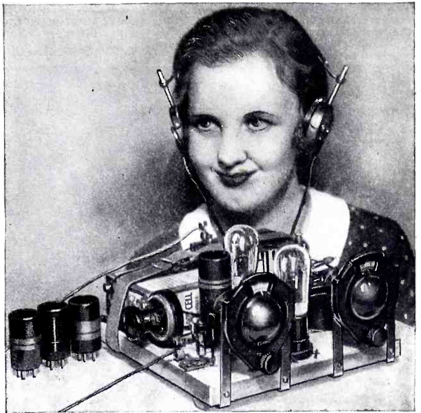
The "Globe-Trotter" in actual operation, with extra plug-in coils at the left.
