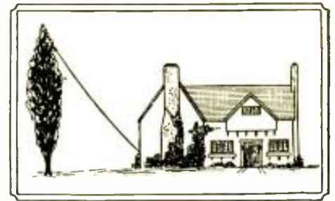
"Vertical" aerials can often be advantageously hung from a tree.
