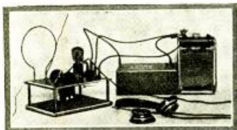
Fig. 8—Complete ultra-short wave receiver for use of head-phones.
