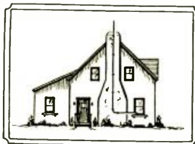
Another happy idea—fasten the vertical antenna to the side of a chimney, supporting the aerial wire on insulators, of course.
