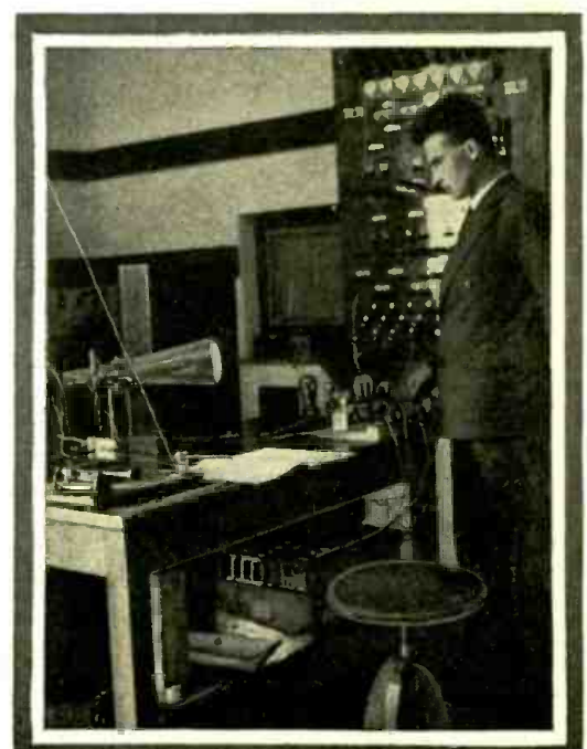
Left—Apparatus used for accurately ascertaining frequencies in the short wave range. A standard quartz crystal having been excited in its upper harmonics, interference is produced with the frequency to be measured.
