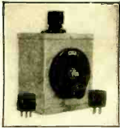
The Delft wavemeter for measuring length of transmitted or received short waves.
