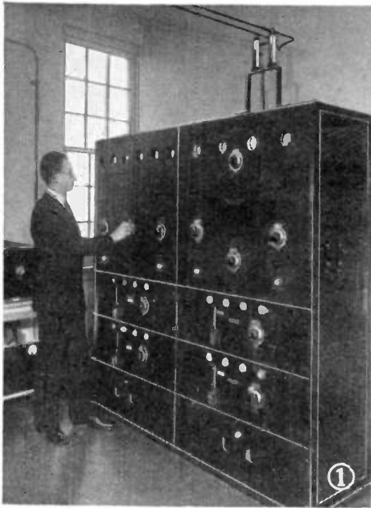
Above—Radio frequency exciter equipment recently rebuilt for W3XAL; Carl Detsch at the controls. Upper right photo shows new 25,000 watt amplifier stage of W3XAL'S powerful class "B" 20 kilowatt modulator at station W3XAL.
