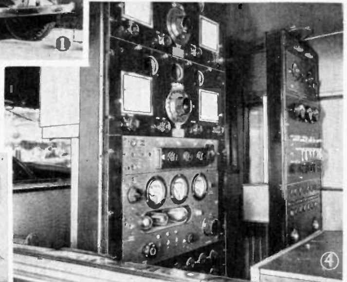
Above—snappy appearing radio "news-gathering" motor car, designated by its owners—the National Broadcasting Company—as their "Mobile unit," which is licensed to transmit on a whole flock of short-wavelengths, which enables the operators to use that wavelength or frequency best suited for the occasion. Fig. 2, below, shows one of the announcers' mikes; Fig. 4, control panels inside the car.
