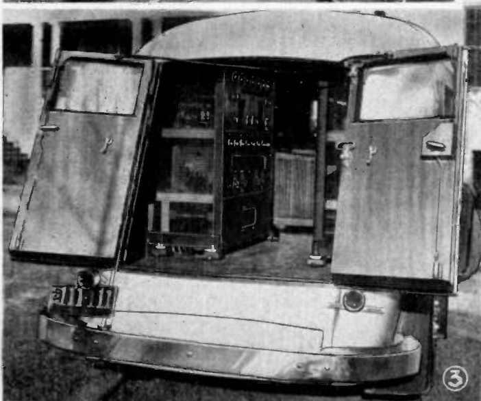
The view above shows separate power plant built into the Mobile transmitting unit, which is used by the N.B.C. to report "spot news" from the scenes of disasters and other happenings. The car is fitted with five short-wave receivers; its most powerful transmitter is rated at 150 watts. This transmitter can project a "news pick-up" a distance of 100 miles when stationary and 50 miles while the car is in motion. Fig. 3 at right, shows rear view of the car with doors opened up. The messages flashed on short-waves from the car are picked up and rebroadcast on the N.B.C. networks. The car can travel 65 to 70 miles an hour and was specially designed for the purpose.
