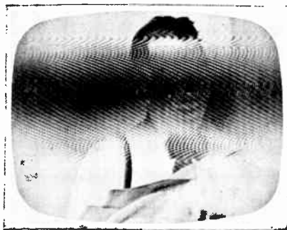
Fig. 5. An example of diathermy interference. Note that the picture has turned negative within the interference band. (Allen B. Du Mont photo)
