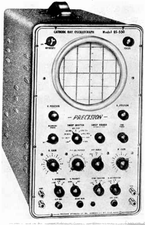
Fig. 1. A cathode-ray oscilloscope useful for television service work. (Precision Apparatus Co. photo)
