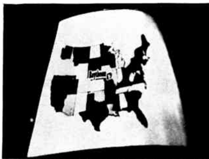
Fig. 15. Distortion of picture caused by a defective yoke. The horizontal coils are influenced more in this case than in Fig. 13. (Raytheon photo)
