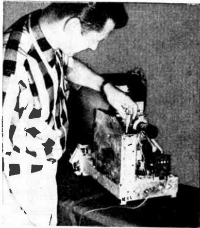
Fig. 2. Removing the horizontal sweep tube from a chassis. This tube along with the high-voltage rectifier and damper are usually located within a cage similar to the one shown
