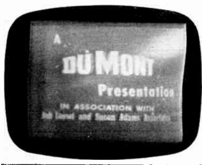
Fig. 18. A low-voltage condition. The picture is undersize and may be dim and blurry. (Allen B. Du Mont photo)
