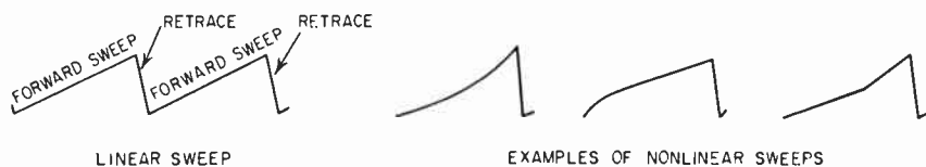
Fig. 11. Graphical representation of good sweep (linear) and examples of nonlinear sweeps. Nonlinear sweep causes the picture to be distorted by compressing or expanding portions of the scene
