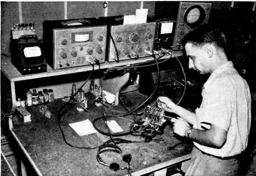
Fig. 13. Aligning a tuner unit. The sweep generator, marker generator, and oscilloscope are used for this purpose. (RCA photo)
