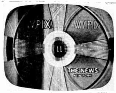
Fig. 1. A bad ghost condition. The dark band is the ghost of the horizontal blanking and sync. (Allen B. Du Mont photo)
