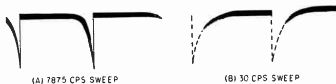
Fig. 5. Sync pulses as they might appear on an oscilloscope. A shows horizontal pulses; B shows vertical pulses
