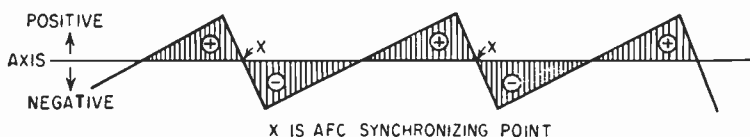
Fig. 6. This waveform shows how a sawtooth voltage disposes itself about an a-c axis. The voltage swings equally from positive to negative
