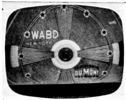
Fig. 14. Vertical distortion of picture caused by a failure in the vertical sweep circuit. (Allen B. Du Mont photo)
