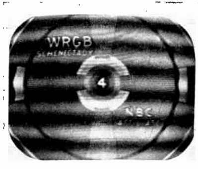
Fig. 2. Noise bars caused by thumping a microphonic video tube. (General Electric photo)
