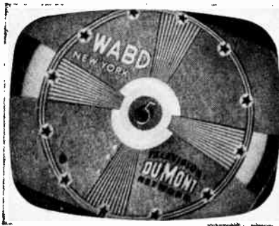
Fig. 15. A tilted picture. This condition is caused by a tilt of the deflection yoke, not by a tilt of the picture tube. (Allen B. Du Mont photo)
