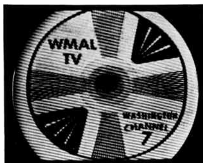
Fig. 6. An example of c-w interference. The lines could be finer or broader or appear at any angle
