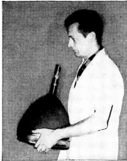
Fig. 5. The proper way to carry a picture tube. It should not be carried by the neck
