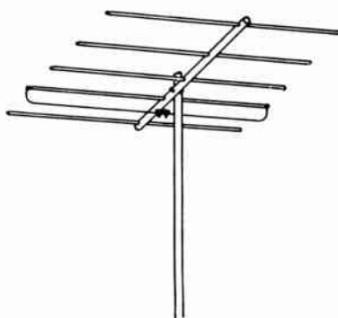
Fig. 2. A typical single-bay Yagi antenna having five elements
