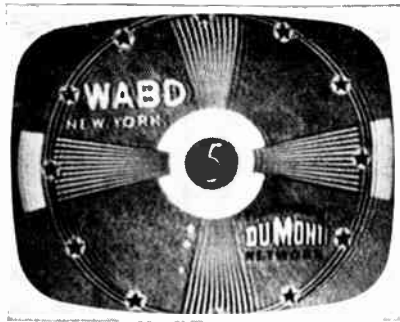
Fig. 4. Transient ghosts, or "ringing." This condition is caused by a defect in the set. (Allen B. Du Mont photo)
