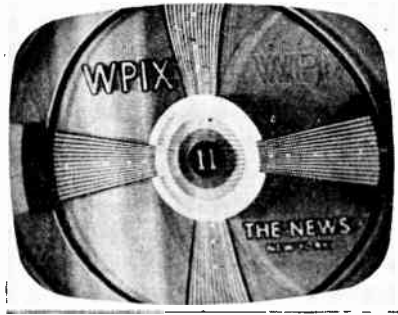
Fig. 2. A negative ghost. Note that blacks and whites are reversed in the ghost. Now the ghost of the horizontal blanking and sync appears as a white band. (Allen B. Du Mont photo)
