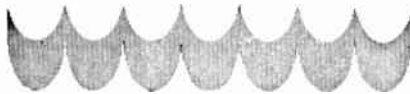
Fig. 16. This sketch suggests the waveform of the combination of horizontal and vertical convergence currents
