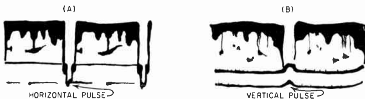
Fig. 4. A video waveform as it appears on an oscilloscope. A shows horizontal pulses because the sweep speed is 7875 cps. B shows vertical pulses because the sweep speed is 30 cps
