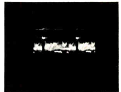
TP2-788 Figure 12. Video Amplifier Plate, Pin 7 66 volts, 60 c.p.s.
