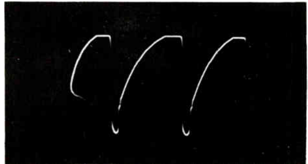
Figure 32. Horizontal-Output Grid, Pin 5 130 volts, 15,750 c.p.s.
