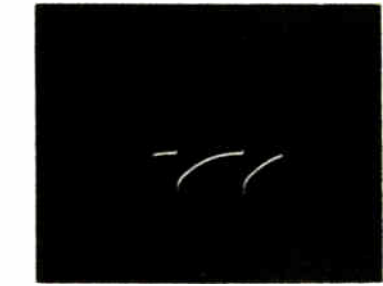
Figure 22. Vertical-Oscillator Grid, Pin 2 170 volts, 60 c.p.s.
