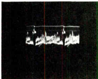
TP2-790 Figure 13. Sync Amplifier Plate, Pin 6 66 volts, 60 c.p.s.
