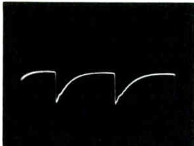
TP1-1095 Figure 28. Horizontal-Amplifier Grid Pin 5* 110 Volts, 15,750 C.P.S.
