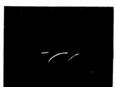
TP2-643 Figure 18. Vertical-Oscillator Grid, Pin 2 165 volts, 60 c.p.s.
