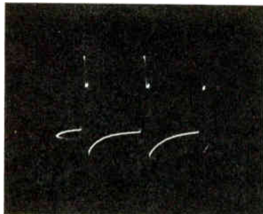
Figure 29. Horizontal-Deflection Yoke, *Pin 7 of J800 3000 volts, 15,750 c.p.s. *See CAUTION note below.
