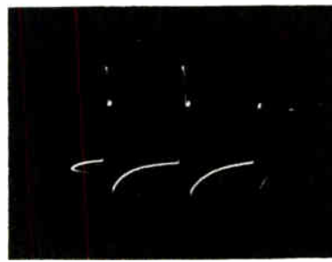
Figure 32. Horizontal Deflection Yoke. *Pin 7 of J800 3000 volts, 15,750 c.p.s. *SEE CAUTION below.
