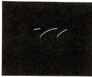
Figure 20. Vertical-Output Grid, Pin 7 120 volts, 60 c.p.s.
