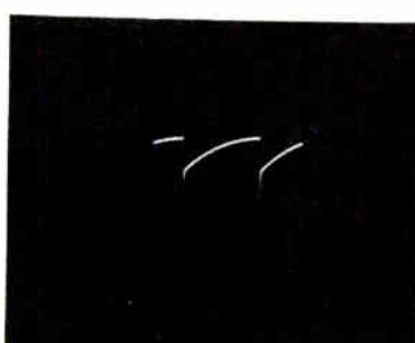
TP2-644 Figure 20. Vertical-Output Grid, Pin 7 120 volts, 60 c.p.s.
