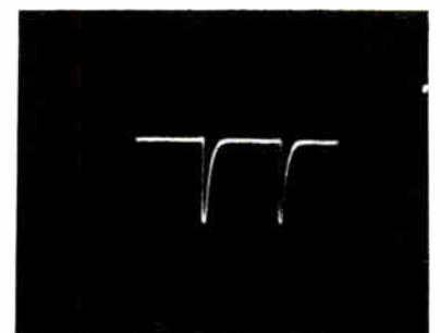
TP2-792 Figure 15. Sync Separator Plate, Pin 5 19.8 volts, 15,750 c.p.s.
