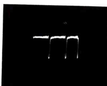
TP2-793 Figure 17. Sync Inverter Cathode, Pin 8 6.8 volts, 15,750 c.p.s.
