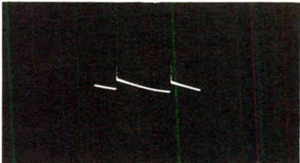
Figure 20. Vertical-Output Plate, Pin 9 450 volts, 60 c.p.s.
