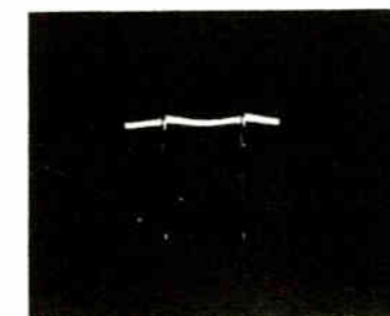
Figure 20. Phase-Splitter Grid, Pin 7 16 volts, 60 c.p.s.
