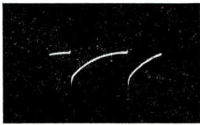
Fig. 13. Vertical-Oscillator Grid, Pin 7, 140 volts, 60 c.p.s.
