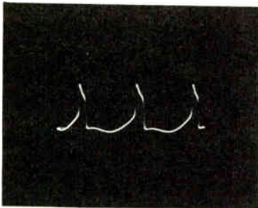
Figure 25. Horizontal Oscillator, Junction of L800, R806, and C806 35 volts, 15,750 c.p.s.
