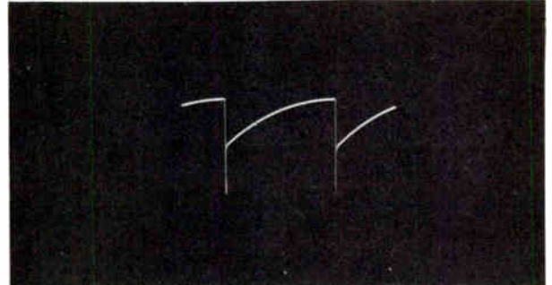
Figure 24. Vertical-Output Grid, Pins 2 and 7 120 volts, 60 c.p.s. TP2-644-A
