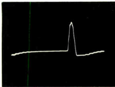
Figure 27. Horizontal-Amplifier Plate,** See CAUTION 5000 Volts 15,750 C.P.S.
