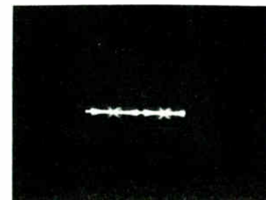
TP2-658 Figure 16. Noise Inverter Cathode, Pin 8 Wave shape and amplitude vary with noise
