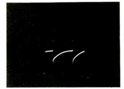
TP2-643 Figure 21. Vertical Oscillator Grid, Pin 2 165 volts, 60 c.p.s.
