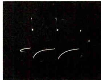
Figure 33. Horizontal-Deflection Yoke, *Pin 7 of J800 5600 volts, 15,750 c.p.s. *See CAUTION above.
