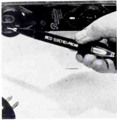
Pencil-type neon tester for checking outlets and determining if voltage is present at fuses, sockets, switches, lines and terminals. (Sico Electro-Probe; Superior Instruments Co., 2435 White Plains Rd., New York 67, N. Y.)
