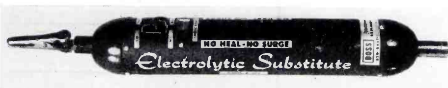
FIG. 1: DOSS MODEL D-600 ELECTROLYTIC SUBSTITUTE shunt-tests an electrolytic filter capacitor without the charging surge normally encountered. Probe-mounted clip at left prevents tester from dangling and supplies necessary negative connection.
