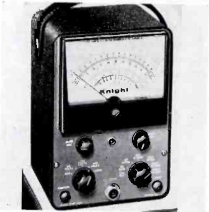
Printed-circuit vtm kit featuring low-leakage switches and film type 1% precision resistors. Seven dc and ac rms ranges are included as well as seven ac peak-to-peak ranges and six resistance ranges. (83 Y 125; Allied Radio Corp., 100 N. Western Ave., Chicago 80, Ill.)
