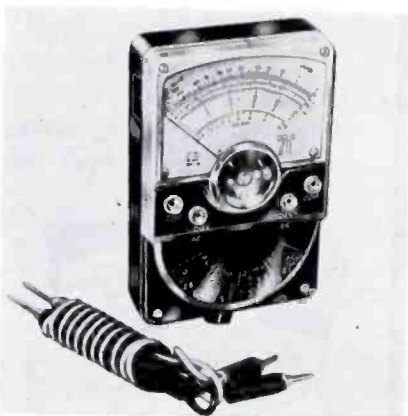
Miniature multitester featuring a 38 micro-amp D'Arsonval movement with jewelled bearings and 23 dc and ac voltage, dc current, resistance and decibel ranges. (AR-660; Argonne Electronics Manufacturing Corp., 165-11 South Rd., Jamaica 33, N. Y.)
