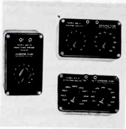
Line of decade boxes which includes three capacitance models, three resistance models and four inductance models. Multiple-dial units have highest value multiplier on left-hand side so that readings are made from left to right. (Distributor Div., Aerovox Corp., New Bedford, Mass.)
