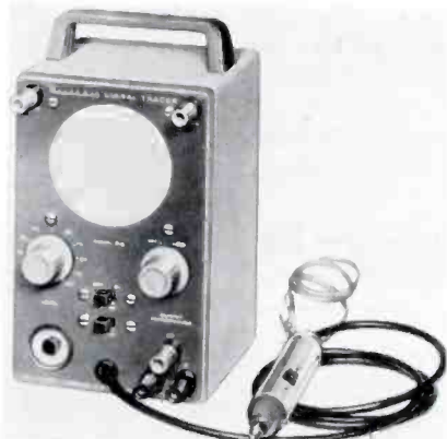
High-gain signal tracer kit for tracing rf, if and audio signals in either tube or transistor AM or FM receivers. Contains a noise locator circuit to permit isolation of noisy and intermittent components. Signal strength is indicated aurally and visually. (T-4 Heath Co., Benton Harbor 11, Mich.)
