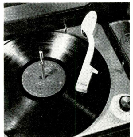
FIG. 3: COMPATIBLE TONE ARM on record changer plays either stereo or monaural records. Cartridge is equipped with 0.7-mil diamond sapphire for LP records and 3-mil sapphire for 78-rpm discs.
