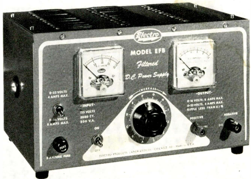
FIG. 1: DC POWER SUPPLY suitable for servicing transistorized and other low-voltage equipment.
