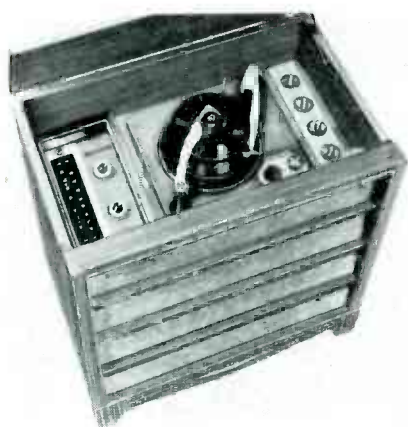
FIG. 1: AM-FM RADIO-PHONO with 16-watt amplifier and 4-speed changer.
