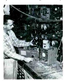
CHECKING TRANSMITTER tuning with a grid-dip meter. The circuit tracer to the right of the marine radiotelephone serves to check receiver circuits.
