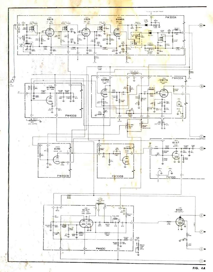
Circuit Diagram of 21-Inch Color-TV Chassis Which Features All-Glass Picture Tube. See Systems Used
