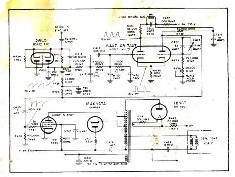
FIG. 2: WESTINGHOUSE horizontal sweep circuit.
