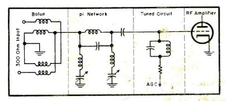
FIG. 1: ANTENNA matching network and its relation to tuner circuitry.
