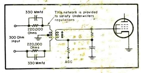
FIG. 2: TYPICAL TUNER input circuit using a matching transformer.
