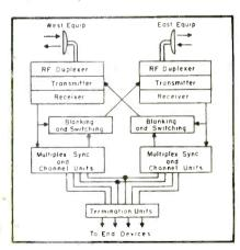
REPEATER with multiplex and termination units. Additional equipment required for this phase of operation is a blanking and switching unit.
