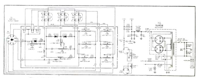
FIG. 6: DYNAMIC CONVERGENCE and power supply circuitry of RCA CTC7 color-TV chassis.
