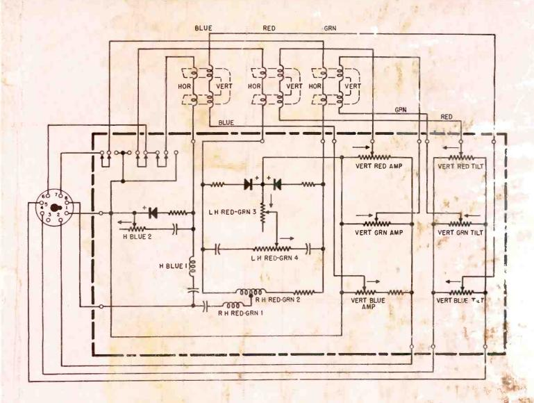
Semiconductor dynamic convergence circuit developed for glass 21-inch tube color-TV receivers.
