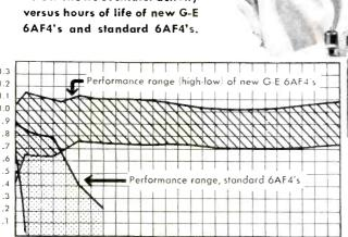
ABOVE: General Electric Design Engineer J. G. Tucker checks, for oscillator activity, new G-E 6AF4 tubes that are undergoing life test. LEFT: Effect of tube operation over long periods on new vs. standard 6AF4's is shown by the chart. Tests of many thousand tubes are represented. Note that the oscillator activity of new G-E 6AFF's averages a straight horizontal line, whereas standard 6AF4's show a sharp, sudden drop . . . meaning rapid loss of picture quality.
