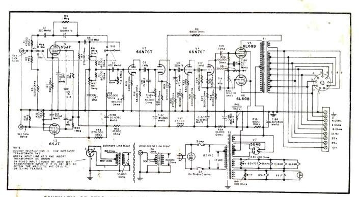
SCHEMATIC OF STROMBERG-CARLSON amplifier included in Trenholm sound-system installation.
