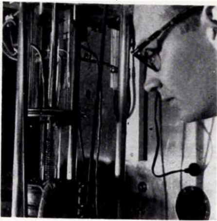
FIG. 1: CHECKING progress of crystal-growing in a resistance-type furnace, the first step in the production of rate-grown transistors; 2,000 transistors can be made from a single crystal ingot.
