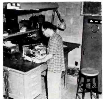
CHECKING tubes on tube testers as well as in the set.
