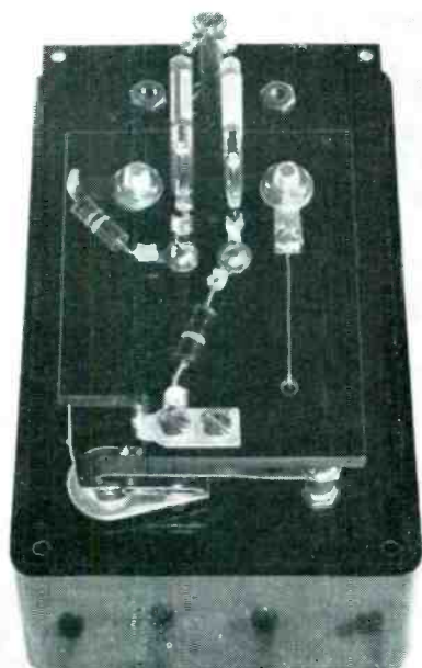
Fig. 4. Interior view of kilovoltmeter. Positive terminal extension is at top center. Resistors extend from it to points on the sub-panel in center; push button, redesigned for adequate spacing, is at lower left.
