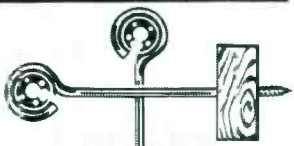
It's a machine screw insulator
