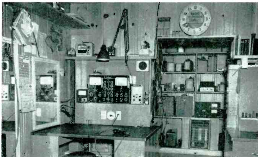
Above and below: The radio and TV benches in the Caldwell service shop. In the racks are the portable test gear used in 2-way work. Some components, tubes and accessories are housed in bench drawers; remainder in racks.
