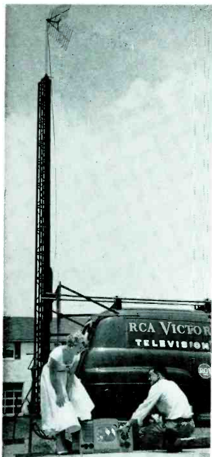
Survey truck with antenna which can be raised up to 70 feet to receive and test signal strength and other data recorded on test receiver shown on ground. (Courtesy RCA)
