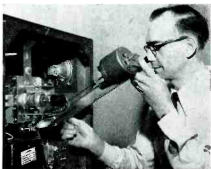
Fig. 5. Installing G.E. translator in TV chassis.
