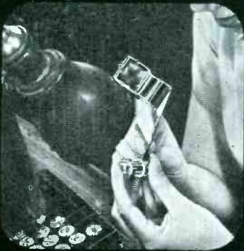
Completed mounts are inspected for visual defects.
