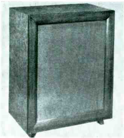
Bass reflex cabinet with mahogany front and matching leatherette top and sides. Single grille cloth covers the entire front panel, concealing the two separate sound openings. Has a 7564-cubic inch capacity for 15-inch speaker. Provided with a 1/2" celulofoam padding. Overall size: 23 3/8" w, 30" h, 14 1/8" deep. (Model DBR-15; Argos Products Co., 310 Main Street, Genoa, Ill.)
