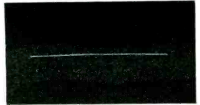
Fig. 5. Trace obtained on 'scope screen when bypassing of common bypass capacitor is complete.
