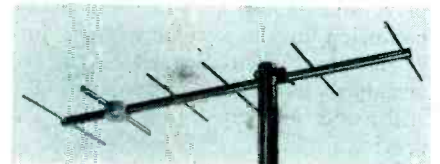
Fig. 8. A six-element yagi probed during the uhf tests.
