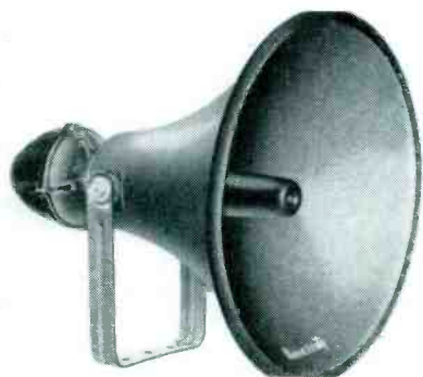
Left and right: Examples of directional and radial-type reflex trumpets used in factories to cover relatively wide areas. Speaker at left features a trumpet and driver*, bell diameters varying from 16 1/4" to 30 3/4" and horn lengths from 12" to 27 1/8". At right is a radial reflex unit**.
