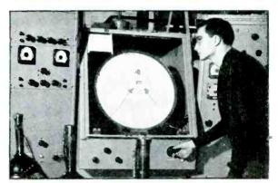
**Every G-E picture tube** is carefully tested for electrical and screen characteristics. Here brightness is being measured, and the screen area inspected for any blemishes. Many other tests follow. G-E tubes are pre-checked for superior performance!
