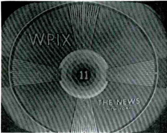
Fig. 2. Patterns with rf interference. Image at left was caused by weak interference from rf , while pattern at left resulted from strong rf -signal interference, providing a picture which has a negative-looking appearance. (Courtesy, Sylvania.*)
