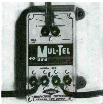
Fig. 3. The two-set coupler which isolates two TV or FM receivers from each other.
