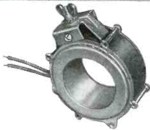
EM-PM FOCUS COIL —These units combine the effects of Alnico 6 permanent magnet and an electromagnet to provide uniform focus with a minimum of circuit power.
