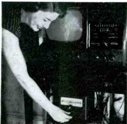
Fig. 8. Application of a booster** ahead of a TV receiver to prevent rf radiation from reaching the antenna.
