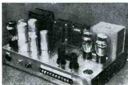
View of 14-watt amplifier designed for custom-built installation.
