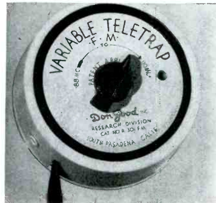
Fig. 9d. Quarter-wave tunable wavetrapp for FM application. (Courtesy Don Good)
