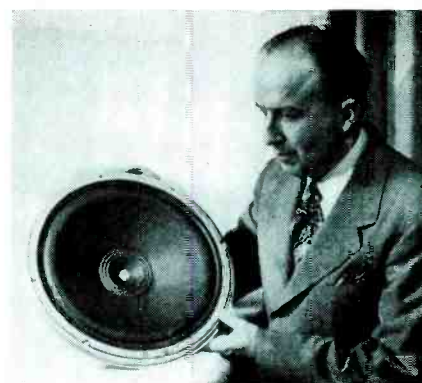
Dr. H. F. Olson of RCA Labs with the duo-cone loudspeaker he developed.
