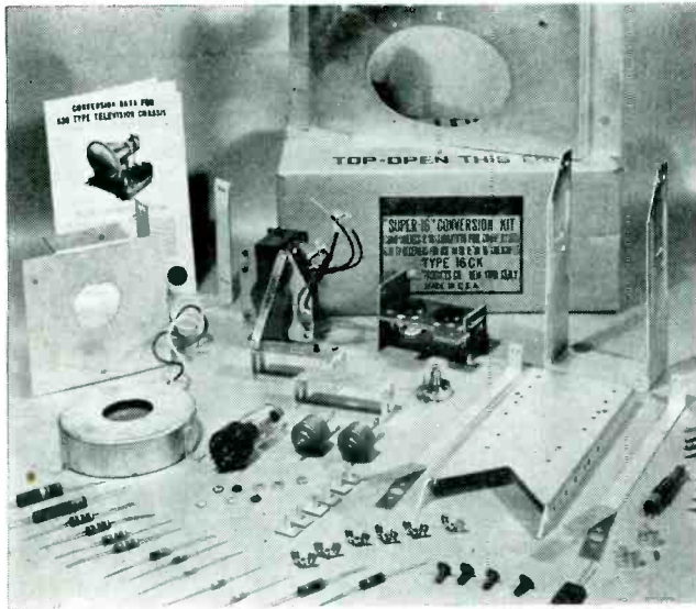
Fig. 2. Assortment of parts supplied in converter kit.
