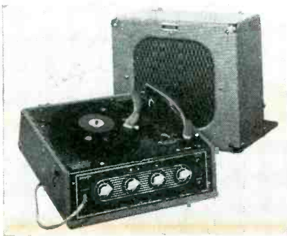
A three-speed player, with a 10 watt amplifier, for 78, 33 \frac{1}{3} and 45 rpm home records and 33 \frac{1}{3} rpm broadcast type recordings. (Courtesy Newcomb Audio)
