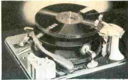
Three-speed automatic phono player. (Courtesy Markel Electric)
