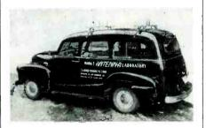
test antennas under all types of transmitting conditions and all urban and rural topographical situations. Equipped with hf signal generators, transmitters, cable, etc.
