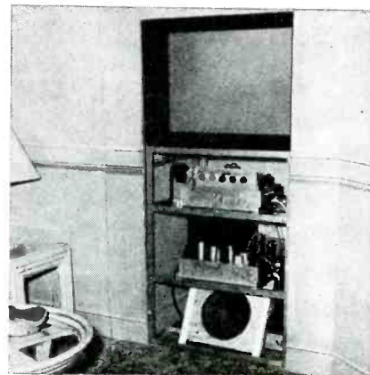
Top: Front view of custom-built projection receiver recently demonstrated by Television Assembly Company. Receiver which provides a 20 x 26 picture uses the Bausch and Lomb refractive arrangements with a F1.9 lens and 5" 5TP4 tube.
