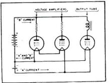
Fig. 1. A typical 3-tube hearing-aid circuit using two voltage amplifiers and an output tube. The *a* supply of 1½ volts feeds two tubes with their .625-volt filaments in series. The filament of the output tube is rated at 1.25 volts. (Courtesy National Carbon Co.)
