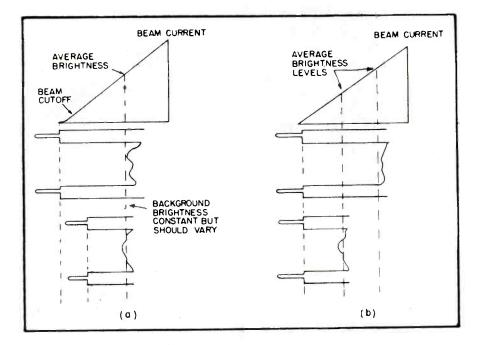
Fig. 3. Signal distribution on grid of picture tube with and without proper restoration. Plot at left shows how the blanking level varies with the signal content. Blanking does not always coincide with the blackout level at all times. The plot at right shows the proper restoration. Here the blanking level is constant and the average bias varies with average brightness of the scene.
