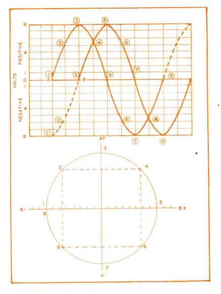
Figs. 4 (above) and 5 (below). The tracing of a Lissajou figure is here shown in detail. Two similar voltages have been applied to both the horizontal and vertical plates. However, one voltage is starting 90°, or  $\frac{1}{4}$  of a cycle later than the other. In Fig. 5, A — and + represent the vertical voltages, and B — and + the horizontal voltages. The position of the dot will then be a function of these two voltages. The resultant picture in this case is a perfect circle.
