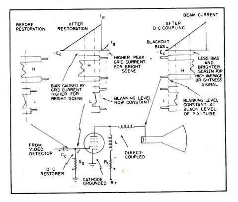
Fig. 4. Grid rectifier type of d-c restorer and waveforms
