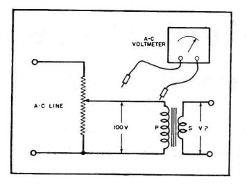
Fig. 1. Dropping voltage to 100 with a potentiometer and measuring circuit to determine winding ratios with an a-c voltmeter.
