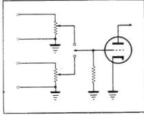
Fig. 1. An input system in its simplest form
