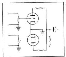
Fig. 3. An input system with pentode highimpedance circuits where isolating resistors are unnecessary.
