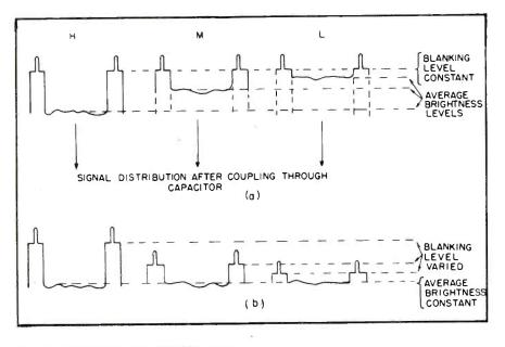
Fig. 2. Loss of average brightness and blanking levels through a coupling capacitor. Upper plot shows the signal distribution after coupling through capacitor.
