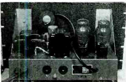
Rear view of rack-mounted amplifier. Shock mountings are at base of chassis.
