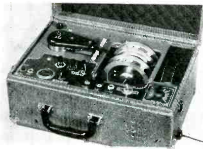
Differential drive unit of a magnetic wire recorder-reproducer. (Courtesy Brush)
