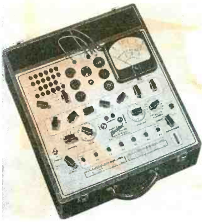
View of tube tester using dynamic mutual conductance circuit.
